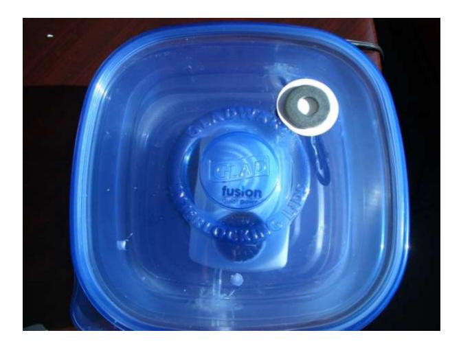
Remove filter after a visible spot develops (hours to days depending on the air quality).
