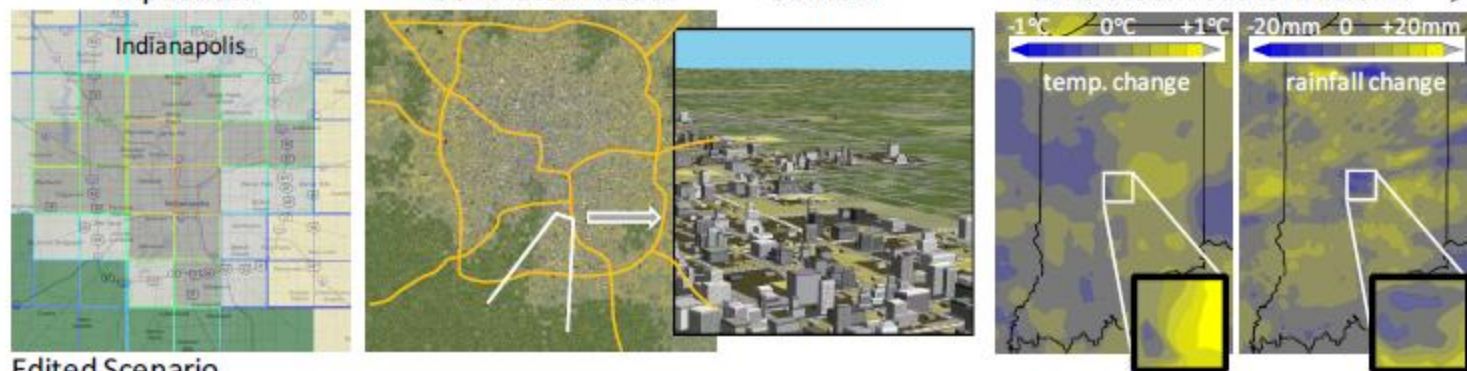
Figure 1. Visualization-based Decision Support System. Top: original urban scenario for Indianapolis, IN. Bottom: hypothetical (edited) urban scenario where the southwest corner became parks. Using LULC data (left column), complemented by population and terrain data, our DSS automatically produces a plausible 3D city model (second and third columns) from which urban morphology parameters are extracted to simulate weather patterns (right column).
