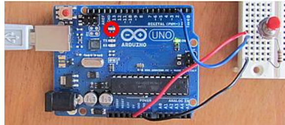
Figure 2. Use a digital pin to read the status of a pushbutton.
