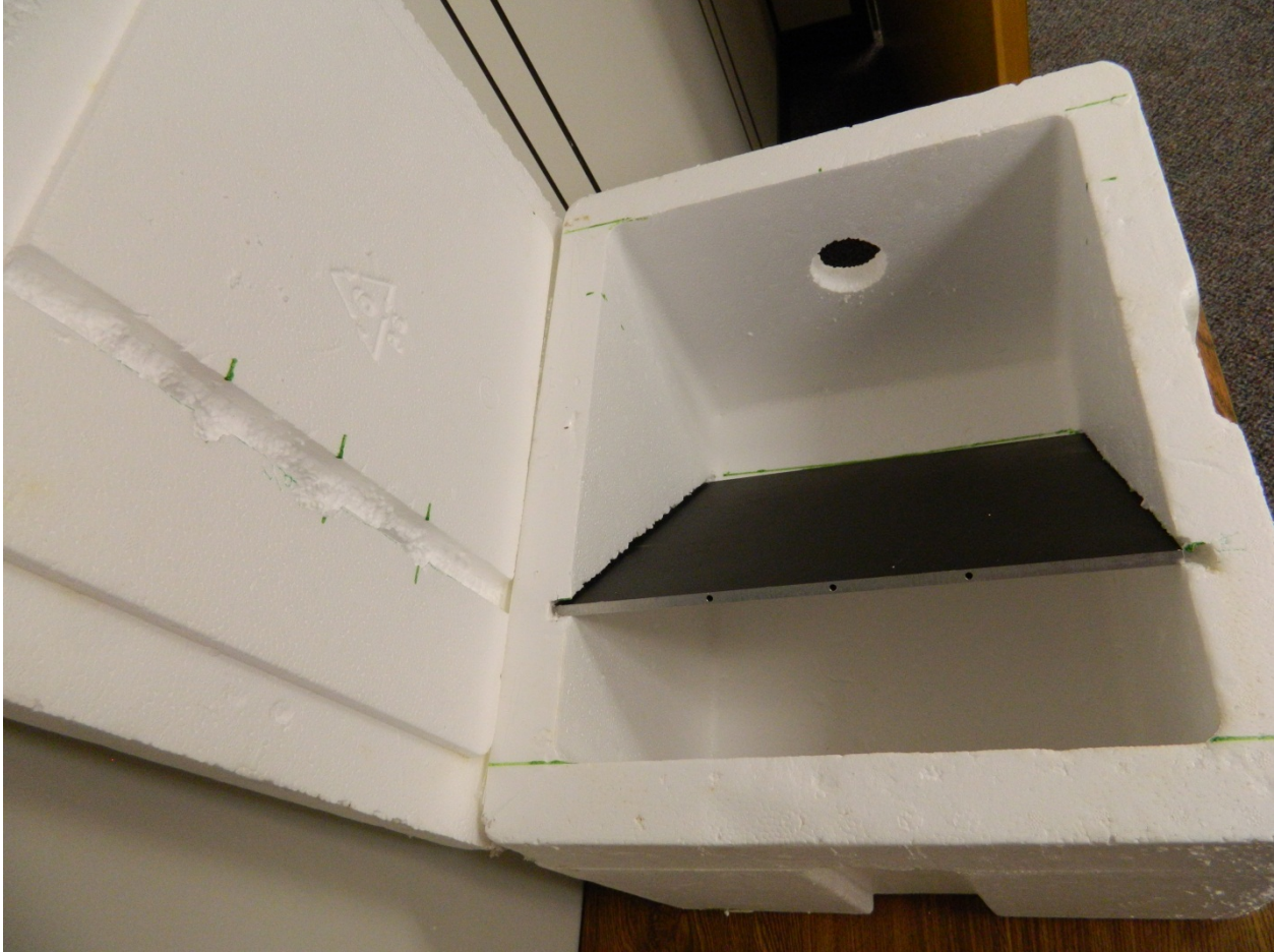
Figure 2.3.3-1. IR calibration fixture made from an ice chest and the calibration plate.
