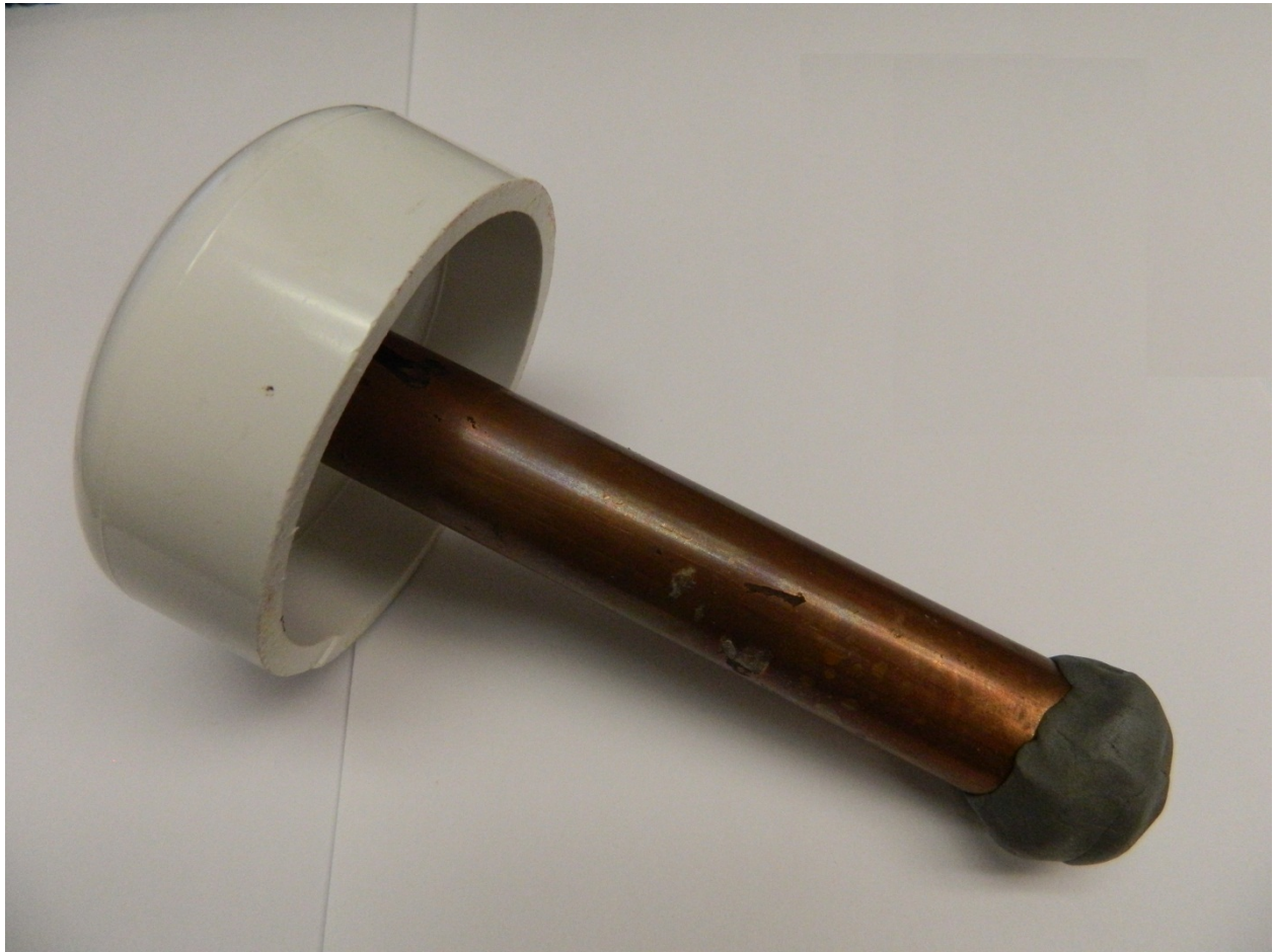
Figure 2.3.2-4. The IR “mini-cavity” for the constant temperature bath.
