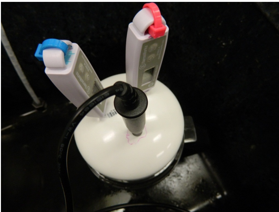
Figure 2.3.2-3. The assembled thermometer intercomparison bath.
