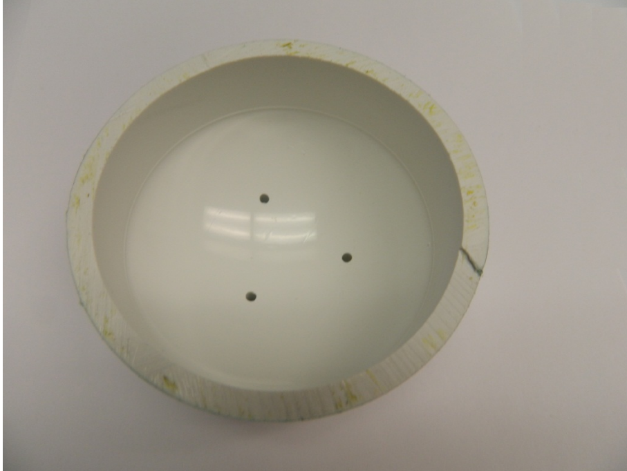
Figure 2.3.2-2. The constant temperature bath cap for thermometer intercomparisons.
