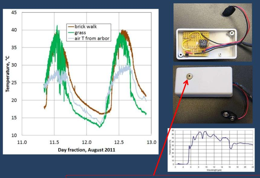
Excelitas TPS 1T 0134 OAA060 calibrated thermopile sensor (~\$20)
